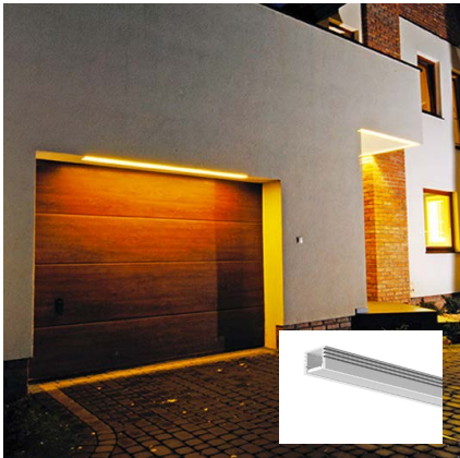
Profil: PDS4 m/ Cover Liger LED-Strip: 24V 12W/M
